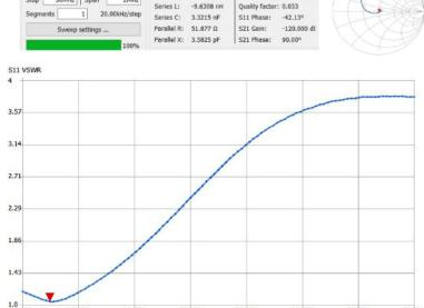
The tuner settings and SWR reading were no different from those obtained during a normal power-on tune-up. This validates the tuning procedure for the QRPp SWR bridge, and confirms that a transmitter is not required antenna tuning.
