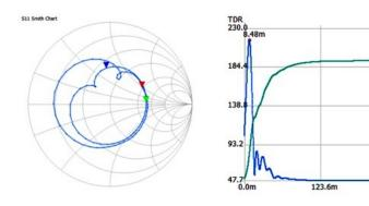
Next the MFJ-969 antenna tuner (or more correctly, the antenna match) is put to work. The following measurements zoom in on the 10-meter band. A single marker is placed near the 10m WSPR frequency. Both the data and the graphics downloaded from the nanoVNA confirm an excellent SWR (less than 1.1).
