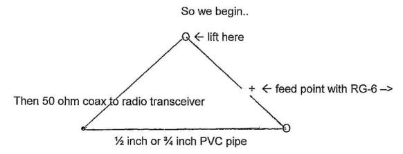
Using colored tape mark a ¼ wave from the end and fold gently - that will be the lifting corner, connecting thru the corner dots with a wave length of AWG 16 wire going thru the pipe then insert one antenna end and RG-6 end into a crimp connector, now the other ends get joined to complete the triangle and you can lift partway to stabliize the lower segment and mark the corners with a band of colored tape to make the next lift guicker.
