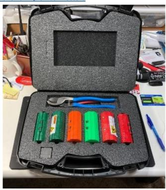
They also sell Amphenol crimp connectors. When the new tools showed up, I made 5 test cables using DXE-8X coax with UHF, BNC and N connectors. I only had one failure out of the 10 connections, and that was all my fault, so I now have a 90% success rate using the new tools on the first try.
