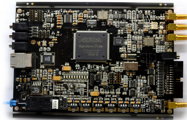
Hermes board. The big square black chip in the center is the FPGA. The only adjustment on the board is a trimmer capacitor at the top, so no more alignment!
